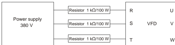
Figure 8-4 380V drive device charging circuit example
